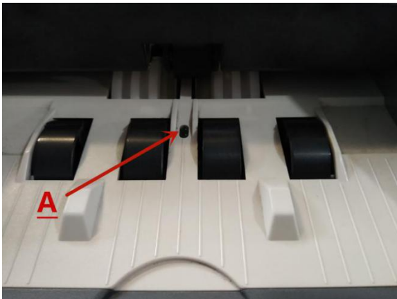
B.Stacker Sensor Error (Something covered the stacker sensor or stacker sensor damaged.)
